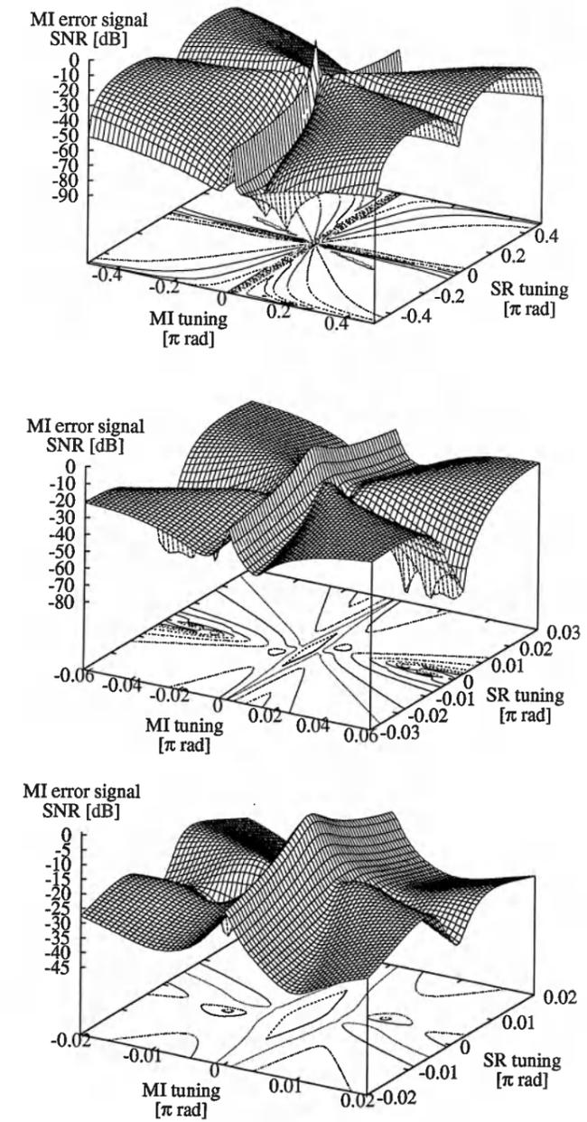
Figure 1.42: The signal-to-noise ratio (in dB) of the Michelson error signal, referred to the SNR at the nominal operating point  $\varphi_{MI} = \varphi_{SR} = 0$ , for small signal frequencies.
