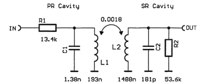
Figure 1.28: An electrical model of coupled resonators. The frequency response of this circuit (for voltages) is exactly identical to the curve shown in Figure 1.26 (with 1% and 2% mirrors). The resonance frequencies of the (undamped) L-C resonators were set exactly identical to the free spectral ranges of the SR cavity and PR cavity, multiplied by two.
