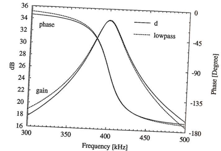
Figure D.2: Approximation of the resonance factor  $d$  by the transfer function of a two-pole low-pass filter around the resonance.
