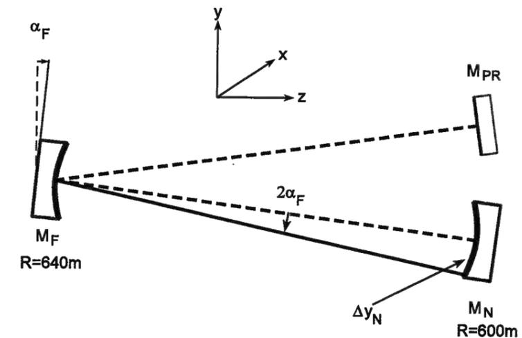
Figure 2.16: Misorientation of  $M_F$  in the GEO 600 PR cavity. The dashed line is the well aligned reference. We have  $\Delta y_N = -\alpha \cdot 1200$  m and no effect on the cavity eigenmode at its waist.
