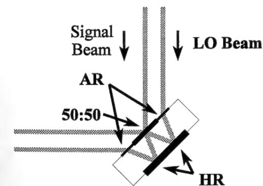
Figure 1.15: Detailed view of the recombination plate. The type of coating in each spot is indicated by 'HR' for high reflectivity, 'AR' for anti-reflection coating, and '50:50' for a semi-reflective beamsplitter coating and symbolized by the linewidth.
