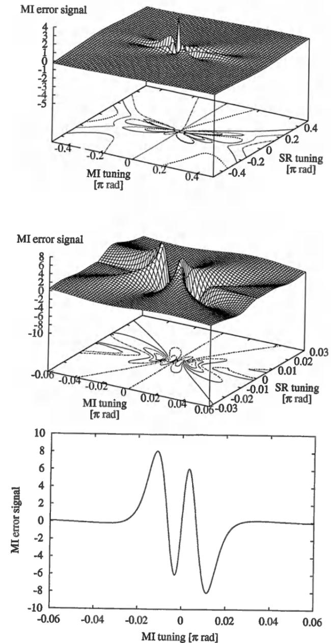
Figure 1.39: Michelson error signal (in arbitrary units) as a function of the tunings  $\varphi_{MI}$  and  $\varphi_{SR}$ , with the PR cavity being kept resonant. The lower curve shows the error signal for  $\varphi_{SR} \equiv 0$ . The tunings  $\varphi_{MI}$  and  $\varphi_{SR}$  are expressed as multiples of  $\pi$  in these plots.
