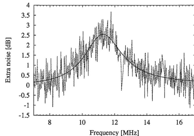
Figure B.5: Measurement of the increased output noise of a tuned photodiode preamplifier caused by a photocurrent approximately equal to  $I_{NE}$ . Shown are the measured data and the curve that was fitted to obtain the photodiode parameters.
