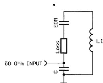
Figure B.10: Alternative resonant transformer circuit with a capacitive voltage divider.
