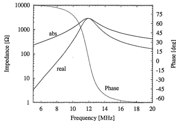
Figure B.4: Impedance of the parallel resonant circuit shown in Figure B.3 for typical values used in the prototype.
