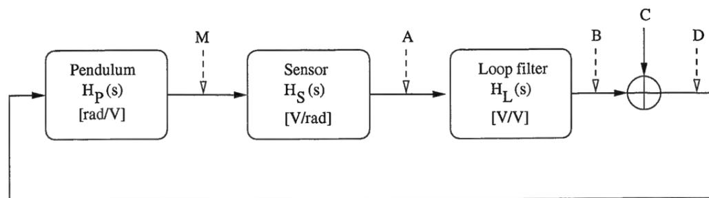
Figure A.13: Simple loop model used for the calibration of the autoalignment system.
