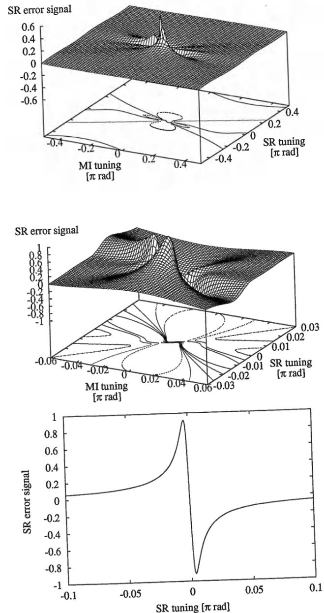
Figure 1.44: SR error signal as a function of the tunings  $\varphi_{\text{MI}}$  and  $\varphi_{\text{SR}}$ , with the PR cavity being kept resonant. The lower curve shows the error signal for the dark fringe state  $\varphi_{\text{MI}} \equiv 0$ . The tunings  $\varphi_{\text{MI}}$  and  $\varphi_{\text{SR}}$  are expressed as multiples of  $\pi$  in these plots.
