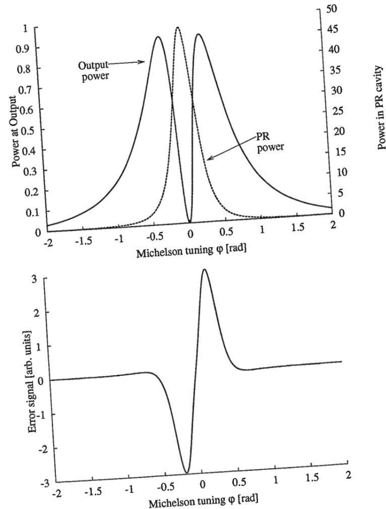
Figure 1.18: Simulation of power recycling in the 30 m prototype. The lower curve shows the Michelson error signal  $H_{1p}$  as a function of the Michelson tuning  $\varphi_{MI}$ . The upper curves show the corresponding DC power at the output and the power buildup in the PR cavity, for unity injected power.
