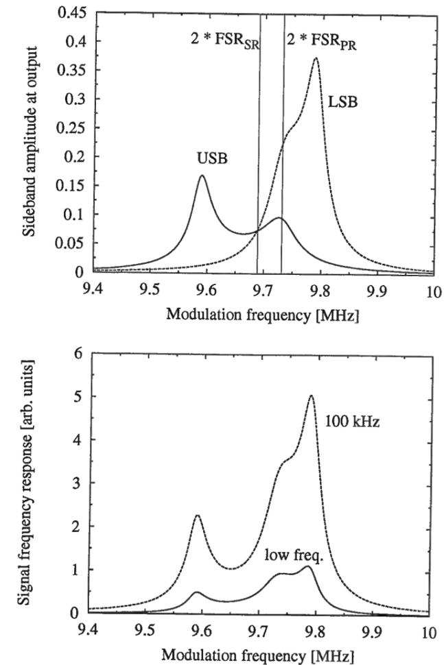
Figure 1.55: Schnupp sideband throughput in detuned dual recycling. The upper plot shows the amplitude of the upper and lower Schnupp modulation sidebands at the output (assuming unity input amplitude). The lower plot shows the dependence of the interferometer frequency response on the Schnupp modulation frequency, for signals of low frequency and 100 kHz, respectively.
