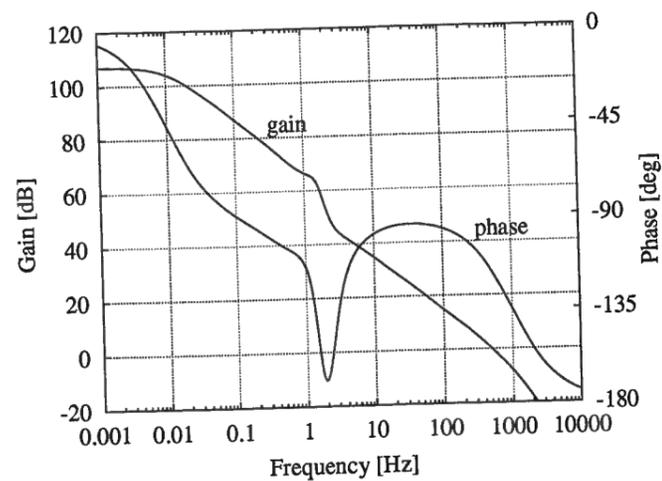
Figure 1.46: Open-loop gain of the SR mirror control loop.
