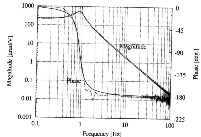
Figure 2.8: Transfer function from the common mode ‘tilt’ input for the end mirrors to the actual tilting motion (measured with PD2). The measured data was fitted to a two-pole low-pass model with  $f_P = 0.90$  Hz and  $Q_P = 2.63$ .
