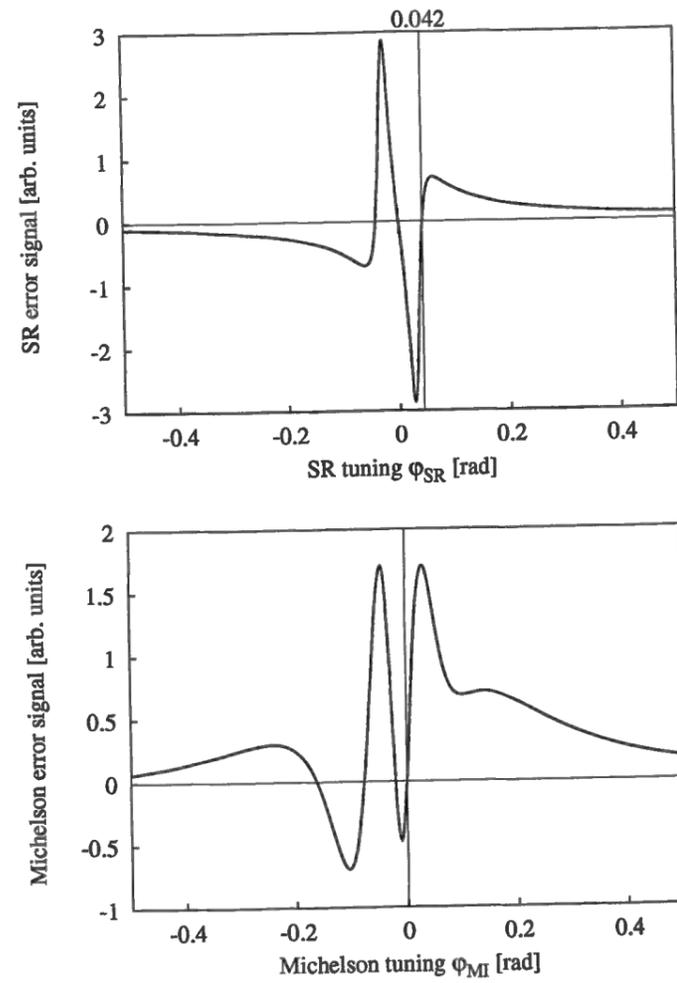
Figure 1.62: Computed error signals for detuned dual recycling, using the parameters that occurred in the experiment (9736 kHz modulation frequency,  $\phi_{SR} = 0.042$  rad,  $\chi_{MI} = -1.65$  rad).
