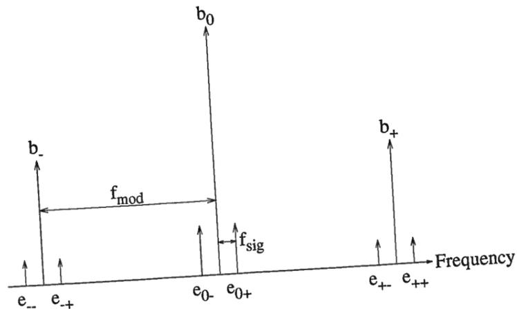
Figure 1.20: The nine light frequencies involved in computing the frequency response.
