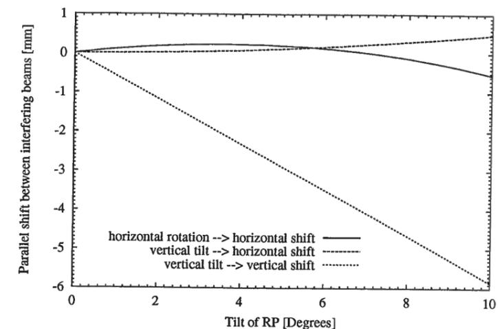
Figure 2.4: Parallel shifts between the two interfering beams in the Mach-Zehnder interferometer caused by a tilt of the recombination plate RP against the beamsplitter BS. The calculations were done assuming a beamsplitter and recombination plate of 3 cm thickness.
