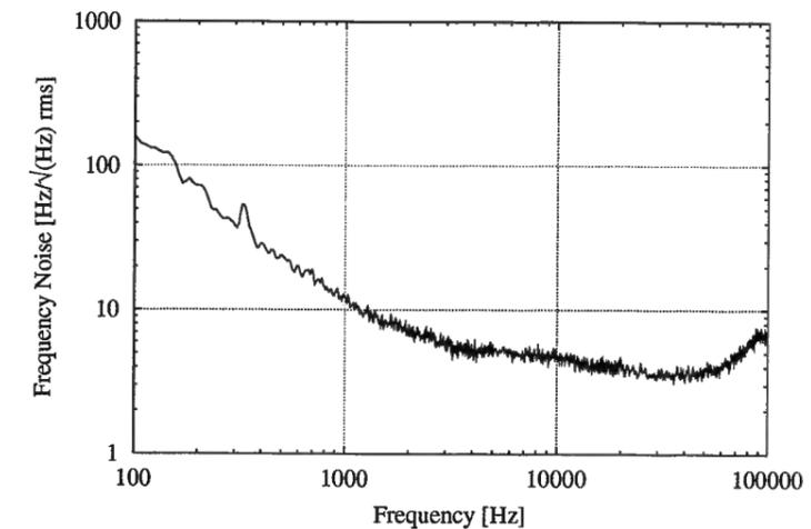
Figure 1.33: Estimated frequency noise of the prestabilized laser (this was *not* directly measured, see text).
