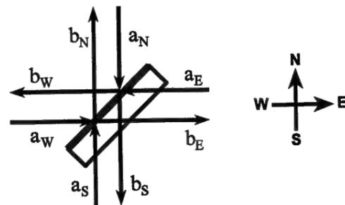
Figure 1.11: Amplitudes at a beamsplitter.
