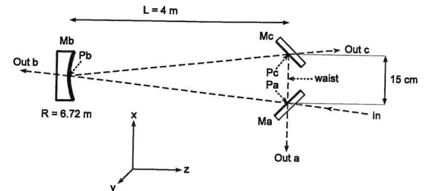
Figure 2.18: Schematic diagram of a GEO 600 modecleaner cavity seen from above.
