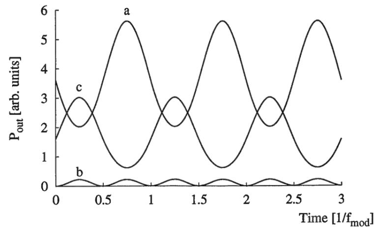
Figure 1.7: The detected power will in general contain a component at the modulation frequency with an amplitude proportional to the phase difference  $\Delta\varphi$ . The curves labelled a, b and c refer to the three operating points shown in Figure 1.6.
