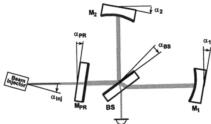
Figure 2.1: Schematic diagram of a power-recycled Michelson interferometer showing all possible angular misalignments  $\alpha$  in one dimension. Beams are shown in their nominal positions, whereas the components are shown misaligned by exaggerated angles.
