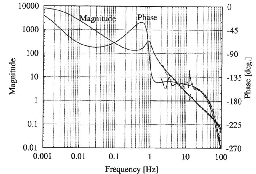
Figure 2.9: Open-loop gain of the Michelson alignment loop. Here the pendulum has  $f_P = 0.9$  Hz and  $Q_P = 3.26$ , and the loop includes a  $f^{1/2}$ -filter active between 1.5 Hz and 45 Hz, an integrator between 3 mHz and 0.3 Hz and a second order low-pass filter ( $f = 85$  Hz,  $Q = 1$ ). Measured data are shown between 2 Hz and 100 Hz, together with the computed extrapolation to lower frequencies.
