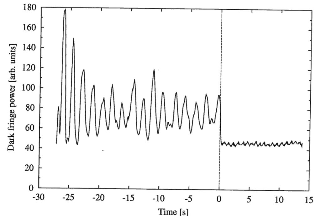
Figure 2.12: Power leaving the dark fringe port of the interferometer (measured with PD3) without and with auto-alignment (switched on at  $t = 0$ ). The final level of 50 units corresponds to about 0.1 ... 0.2% of the power at the beamsplitter.
