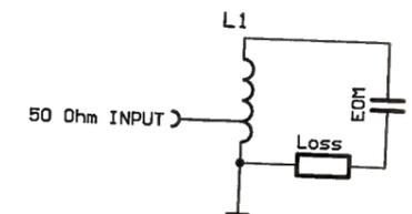
Figure B.9: Alternative resonant transformer circuit with an autotransformer.
