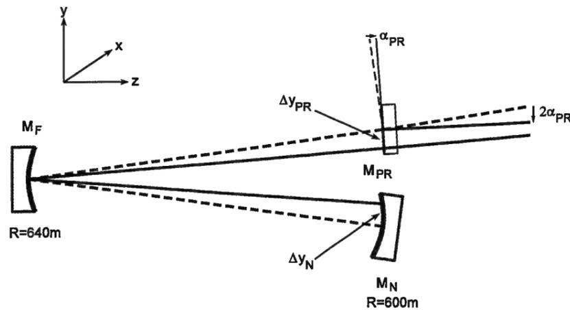
Figure 2.14: Misorientation of  $M_{PR}$  in the GEO 600 PR cavity. The dashed line is the well aligned reference. We have  $\Delta y_{PR} = -\alpha \cdot 600$  m,  $\Delta y_N = \alpha \cdot 600$  m and  $\theta_{PR}^w = 20.7^\circ$ .
