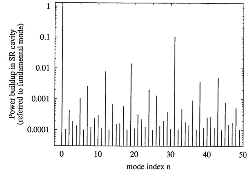
Figure 1.52: Suppression of higher order transversal modes in the signal recycling cavity of the prototype.
