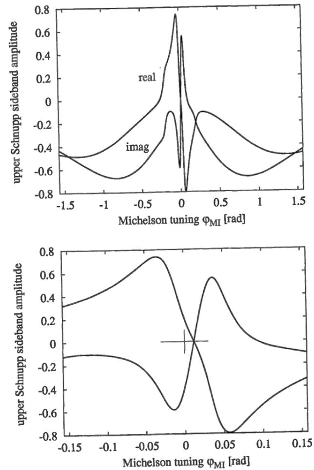
Figure 1.38: Throughput of the upper Schnupp sideband from the EOM to the South port for the 30 m prototype with dual recycling, referred to unity input amplitude. The lower curve shows the central part of the upper curve. The corresponding curves for the lower Schnupp sideband are similar, but mirrored at the  $y$ -axis  $\varphi_{MI} = 0$ .
