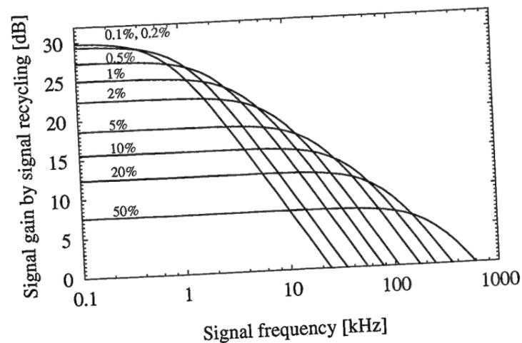
Figure 1.23: Signal gain obtainable in the 30 m prototype by signal recycling, compared against the signal without  $M_{SR}$ . The numbers printed are the power transmissions  $\tau_{SR}^2$  of  $M_{SR}$ . It is assumed that the local oscillator (Schnupp modulation sidebands) is the same for each curve.
