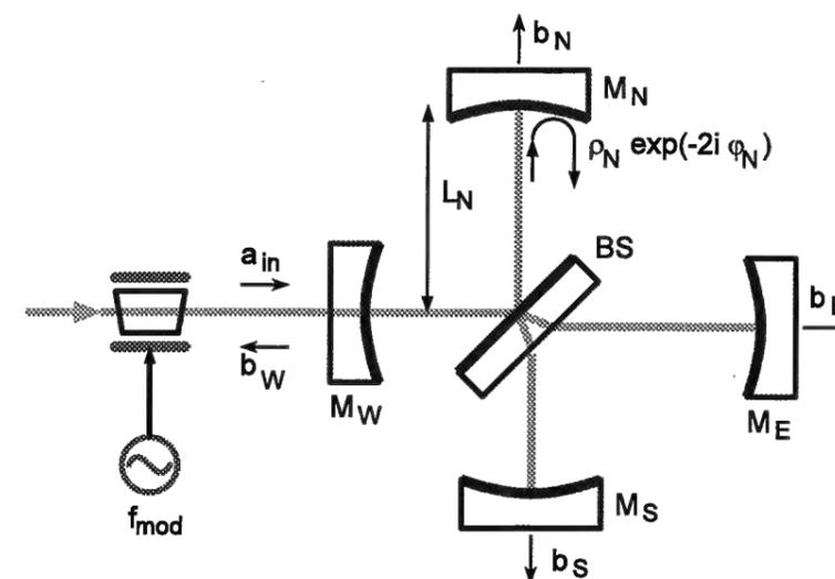
Figure 1.17: The dual recycling interferometer simulated by Jun's program. For simplicity, the arm length  $L$ , mirror reflectivity  $\rho$  and tuning  $\varphi$  are symbolically shown only for the north arm, but are similarly present in the other arms as well.
