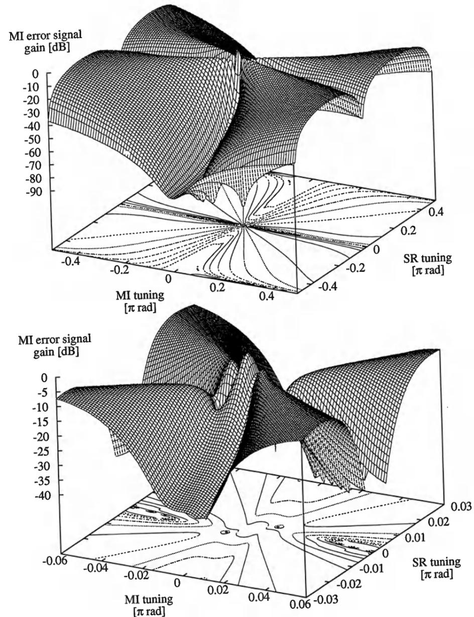
Figure 1.40: The gain (in dB) of the Michelson error signal, referred to the gain at the nominal operating point  $\varphi_{\text{MI}} = \varphi_{\text{SR}} = 0$ , for small signal frequencies.
