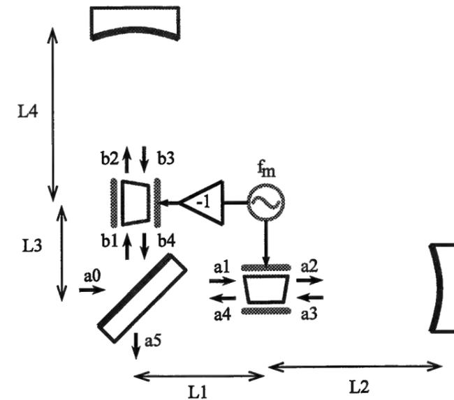
Figure 1.12: A Michelson interferometer with internal modulation. The light amplitudes  $a_0 \dots a_5$  and  $b_1 \dots b_4$  are shown, as well as the lengths  $L_1 \dots L_4$ . The two Pockels cells are driven in anti-phase from the modulation oscillator at the frequency  $f_m$ .
