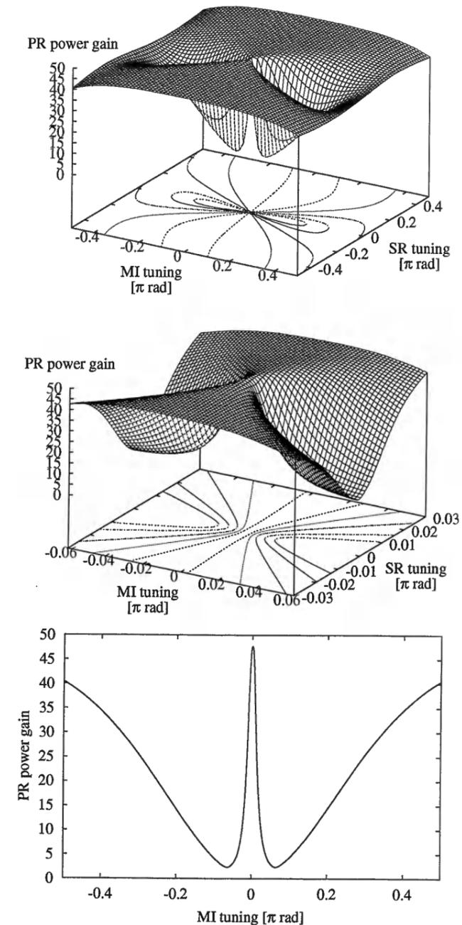
Figure 1.47: Power buildup in the PR cavity (sum of the power in the East arm and the power in the North arm for unity input power) as a function of the tunings  $\varphi_{MI}$  and  $\varphi_{SR}$ , with the PR cavity being kept resonant. The lower curve shows the power for  $\varphi_{SR} \equiv 0$ . The tunings  $\varphi_{MI}$  and  $\varphi_{SR}$  are expressed as multiples of  $\pi$  in these plots.
