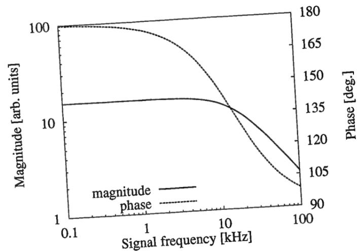
Figure 1.19: Frequency response of the Michelson error signal of the dual recycled 30 m prototype.
