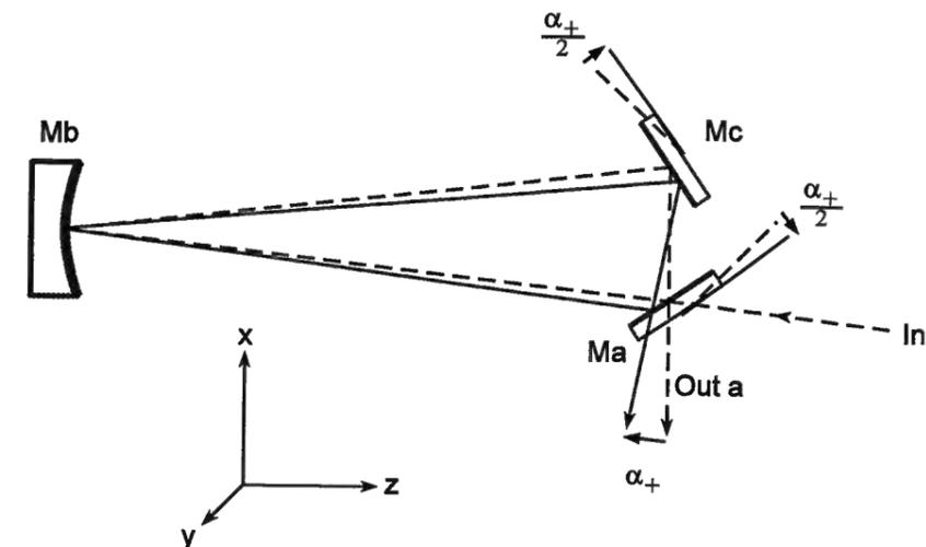
Figure 2.20: Modecleaner with misorientation of  $\alpha_+$ . The dashed line is the well aligned reference. The main effect is a downwards motion of the outgoing beam  $\text{Out}_a$ .
