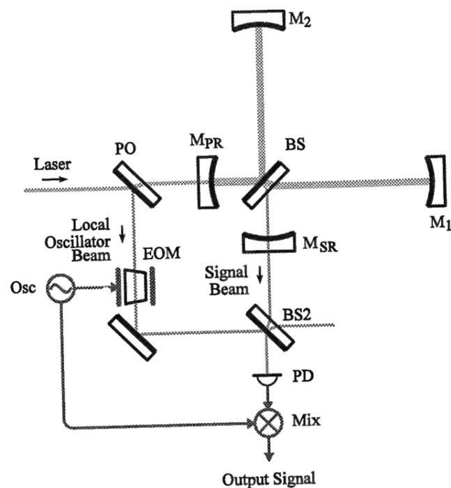
Figure 1.13: Schematic diagram of external modulation. The local oscillator beam is taken from the injected light.
