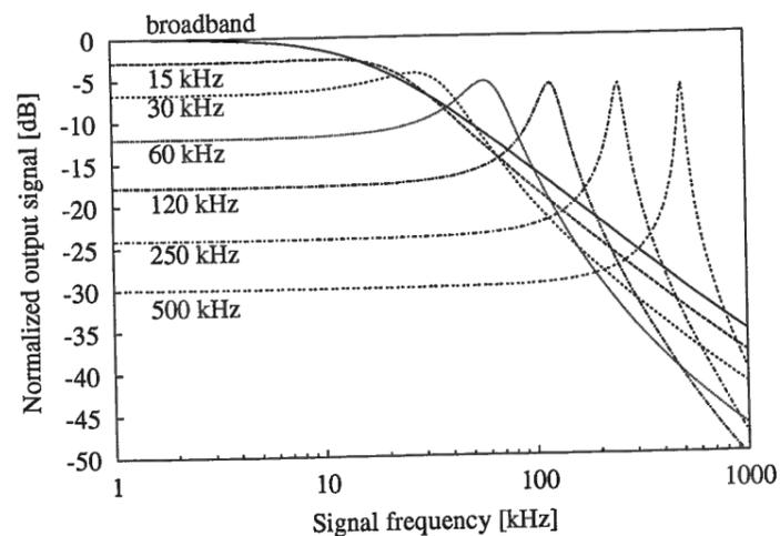
Figure 1.56: Normalized transfer functions of the dual recycled 30 m prototype for various detunings  $\varphi_{SR}$ . For the peak frequencies shown, the corresponding detunings were computed using Equation (1.108), e.g.  $\varphi_{SR} = 0.324$  for  $f_{det} = 500$  kHz.
