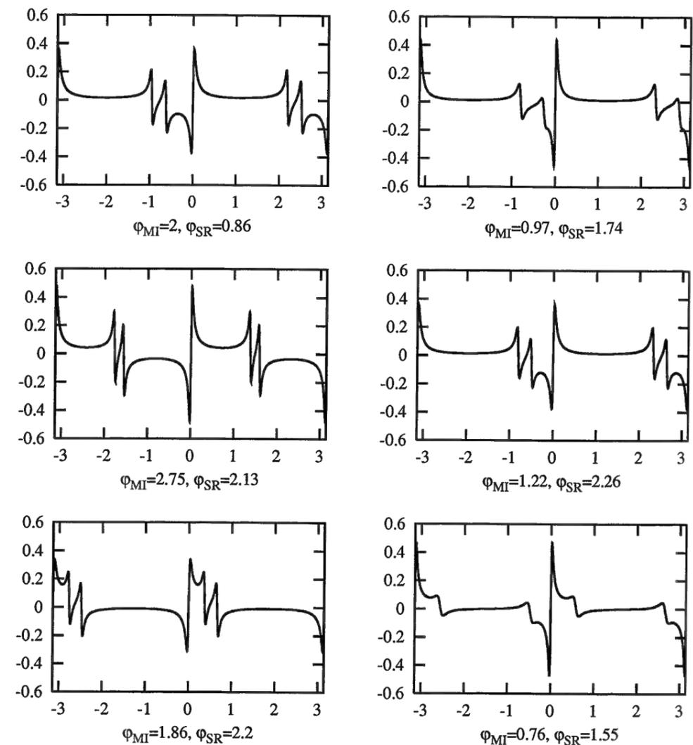
Figure 1.31: PR cavity error signal at six random operating points of the Michelson (tuning  $\varphi_{MI}$ ) and SR mirror (tuning  $\varphi_{SR}$ ). The  $x$ -axis in these plots is the PR mirror tuning  $\varphi_{PR}$  with an offset such that the desired resonance is at zero.
