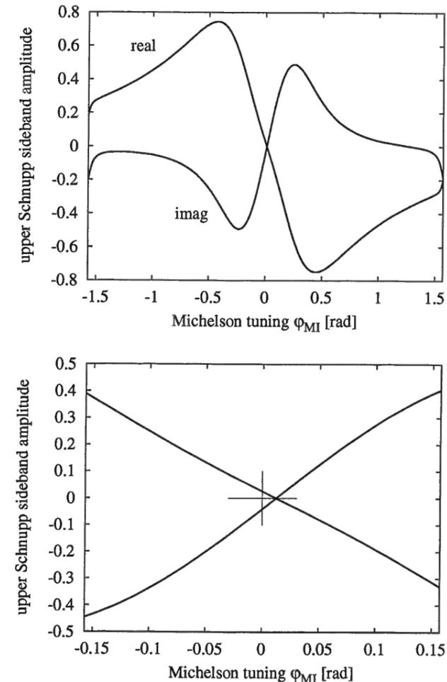
Figure 1.36: Throughput of the upper Schnupp sideband from the EOM to the South port for the 30 m prototype *without* signal recycling, referred to unity input amplitude. The lower curve shows the central part of the upper curve. The corresponding curves for the lower Schnupp sideband are similar, but mirrored at the  $y$ -axis  $\varphi_{\text{MI}} = 0$ .
