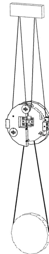
Figure A.3: Sketch of a double pendulum as it is used to suspend the beam-splitter in the prototype.
