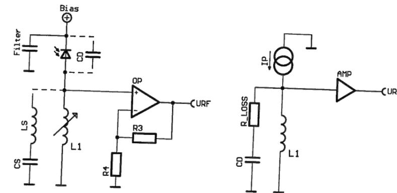
Figure B.3: Basic circuit of a tuned photodiode preamplifier, together with its RF equivalent circuit. The capacitance  $C_D$  represents the photodiode capacitance, whereas the optional series resonant circuit formed by  $C_S$  and  $L_S$  can be used to suppress signals at another unwanted frequency.
