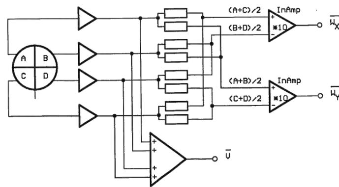
Figure 2.7: Low frequency signal paths in the quadrant detector. ‘InAmp’ are instrumentation amplifiers. The ‘ $\bar{V}$ ’ output is used for monitoring, while the  $\bar{W}_X$  and  $\bar{W}_Y$  outputs are used as error signals for the auxiliary beam steering devices.
