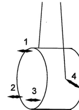
Figure A.5: The approximate physical locations of the four sensors/actuators of each local control channel. The arrows symbolize the directions in which motions are sensed and forces applied.
