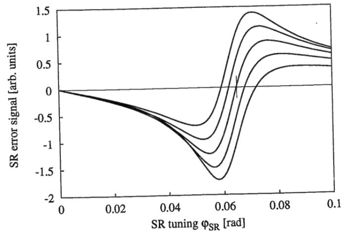
Figure 1.59: SR error signals as a function of the demodulation phase  $\chi_{SR}$ . The five curves shown were computed with offsets of  $-0.5$ ,  $-0.25$ ,  $0$ ,  $+0.25$  and  $+0.5$  rad referred to the demodulation phase  $\chi_{SR}$  used in Figure 1.57.
