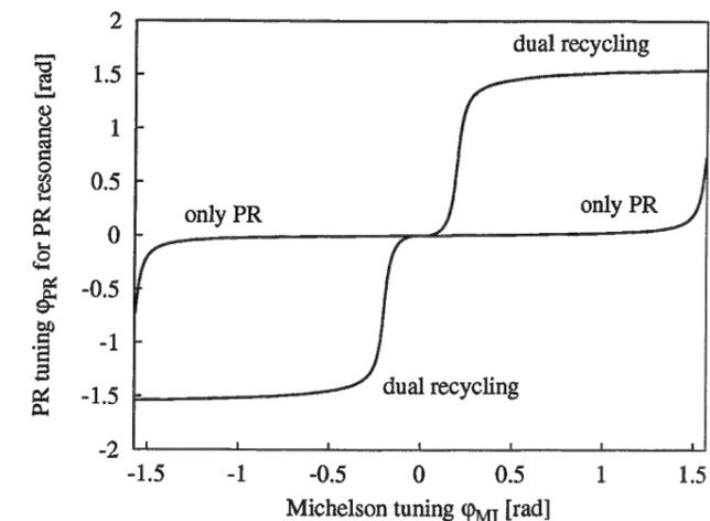
Figure 1.35: The PR cavity tuning  $\varphi_{PR}$  that is necessary to make the PR cavity resonant.
