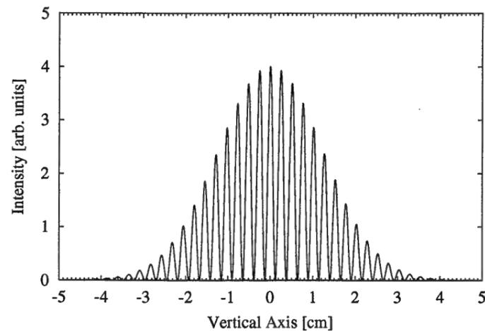
Figure 2.17: Predicted interference structure on the far mirror  $M_F$  of the GEO PR cavity. The intensity along a vertical line through the center of the mirror is shown. The separation between the fringes is 2.55 mm.
