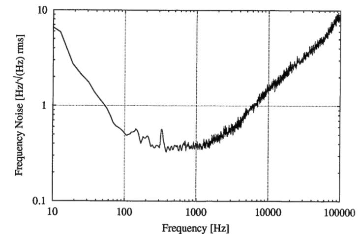
Figure 1.34: Frequency noise (laser frequency referred to PR cavity) with first and second loop in operation.
