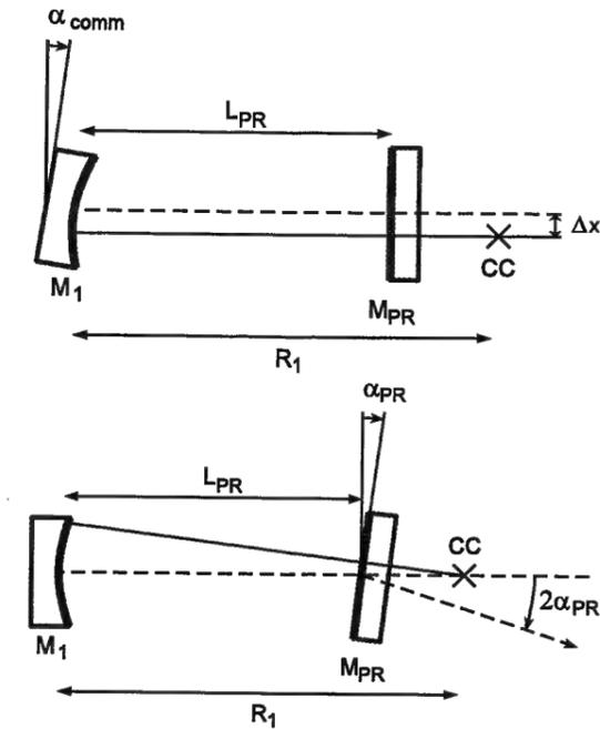
Figure 2.2: Two types of misalignments of the PR cavity. CC denotes the center of curvature of the end mirror(s), with radius of curvature  $R_1$ . The solid line that is orthogonal to  $M_1$  and passes through CC is the axis of the cavity eigenmode.  $L_{PR}$  is the length of the PR cavity. In our prototype,  $L_{PR} \approx 31$  m and  $R_1 = 33$  m.
