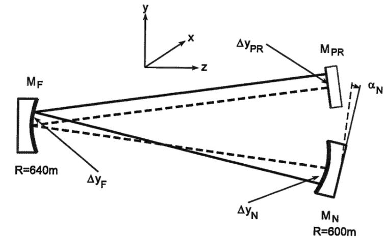
Figure 2.15: Misorientation of  $M_N$  in the GEO 600 PR cavity. The dashed line is the well aligned reference. We have  $\Delta y_{PR} = \alpha \cdot 600$  m,  $\Delta y_F = \alpha \cdot 600$  m,  $\Delta y_N = -\alpha \cdot 525$  m and  $\theta_N^w = 0^\circ$ . The angle between the reference and the misaligned beam between  $M_F$  and  $M_N$  is  $1.875\alpha$ .
