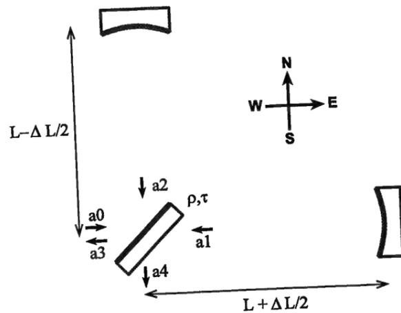
Figure 1.24: A Michelson interferometer with an armlength difference  $\Delta L$ . The incoming beam  $a_0$  is split into two parts. When they return from the two arms (as  $a_1$  and  $a_2$ ), a phase difference has evolved between them. After recombination at the beamsplitter, new beams  $a_3$  and  $a_4$  are formed.
