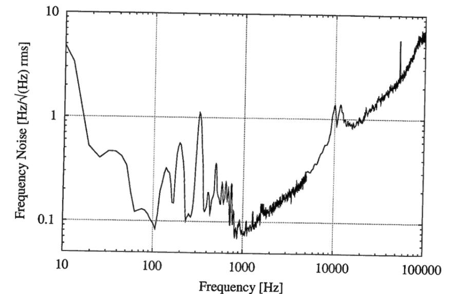
Figure A.12: Frequency noise of the laser light with respect to the power recycling cavity, with the interferometer locked in broadband dual recycling mode.
