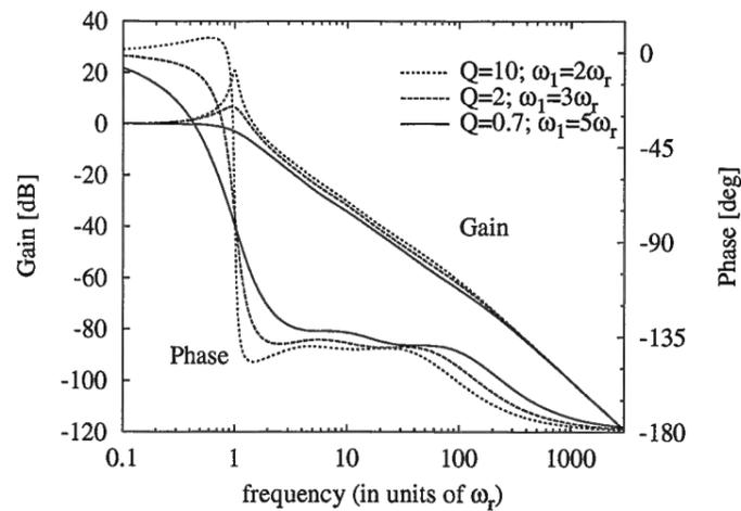
Figure B.16: Computed frequency response of resonant systems together with the  $f^{+1/2}$  filter.
