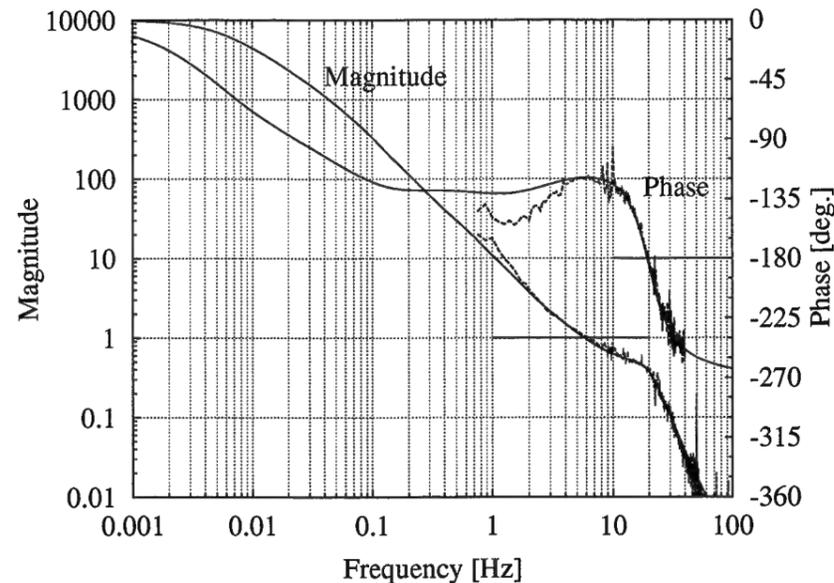
Figure 2.10: Open-loop gain curve of the end mirror common mode alignment loop ( $y$ -channel). The pendulum resonance is electronically compensated by a biquadratic filter that introduces the new pole at 20 Hz with  $Q_{\text{pole}} = 1.5$ , an integrator starts at 5 mHz, and there is a  $f^{-1/2}$  filter active between 80 mHz and 2.5 Hz. Measured data are shown between 0.75 Hz and 100 Hz, together with the computed extrapolation to lower frequencies.
