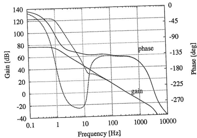
Figure 1.43: Open loop gain of the Michelson dark fringe lock, for a typical unity-gain frequency of 300 Hz. The dashed curves show the open-loop gain with the additional DC gain active.
