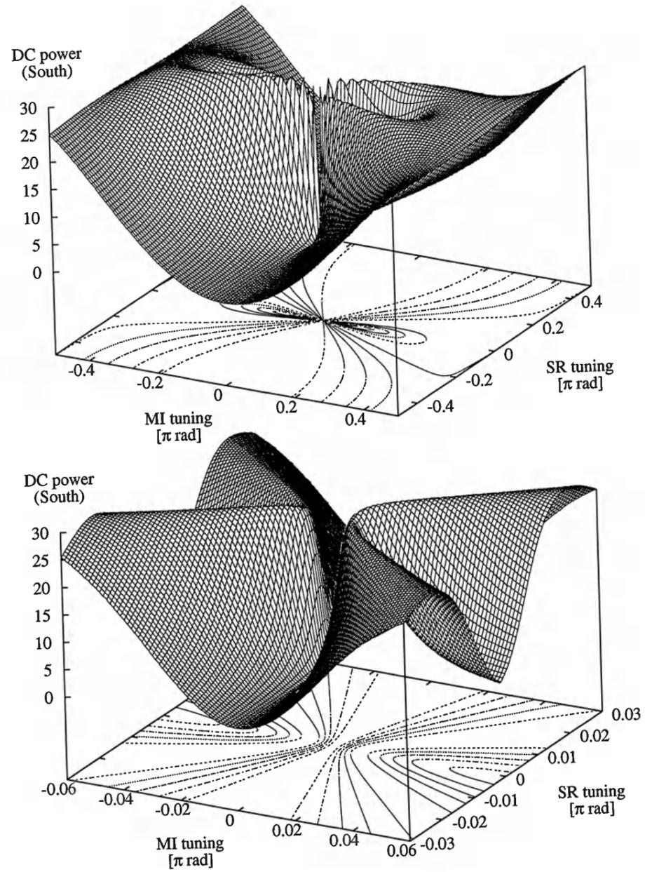
Figure 1.41: The DC (average) light power arriving at the photodetector, referred to unity at the nominal operating point. Note that this diagram was computed from  $H_0$  (Equation (1.49)) and therefore includes the power due to the Schnupp sidebands.
