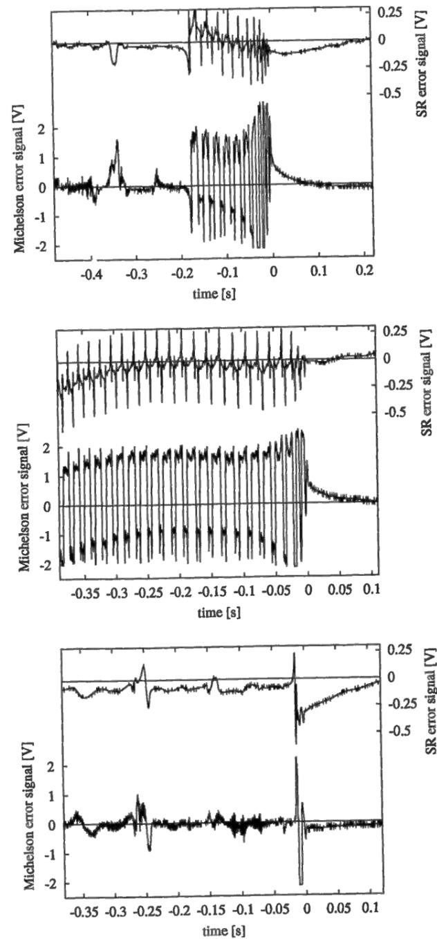
Figure 1.48: Some lock acquisition transients recorded in the dual-recycled 30 m prototype. The time axis has been shifted such that  $t = 0$  corresponds to the approximate time of lock acquisition.
