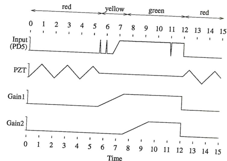
Figure B.12: Sketch of important signals in the automatic lock acquisition circuit and of the corresponding color-coded states. The time-scale is arbitrary.
