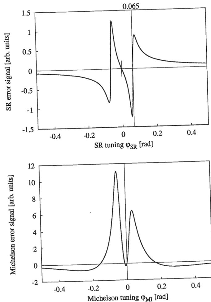
Figure 1.57: Error signals for detuned dual recycling (see text). The nominal operating point is indicated by the long thin lines.
