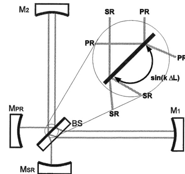
Figure 1.25: Symbolic representation of a dual recycled interferometer with armlength difference  $\Delta L$  in the dark-fringe condition. For the carrier, PR cavity and SR cavity are independent in this idealized model. For light of other frequencies ( $k \neq 0$ ) there is a coupling between these cavities. Beams in the long arms are shown spatially separated, although in reality they are superimposed.
