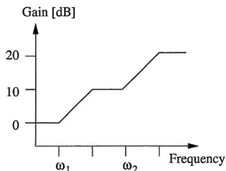
Figure B.14: Straight-line approximation of the desired frequency response for the  $f^{+1/2}$  filter ( $\omega_2 = 10\omega_1$ ).
