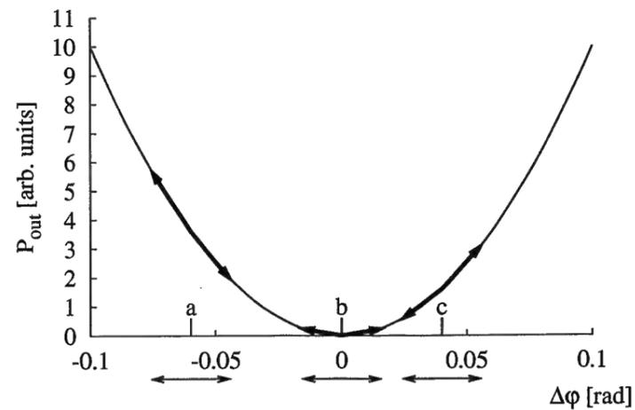
Figure 1.6: When the phase difference is modulated periodically, the output power will change in the rhythm of the modulation. Three different operating points a, b and c are shown.
