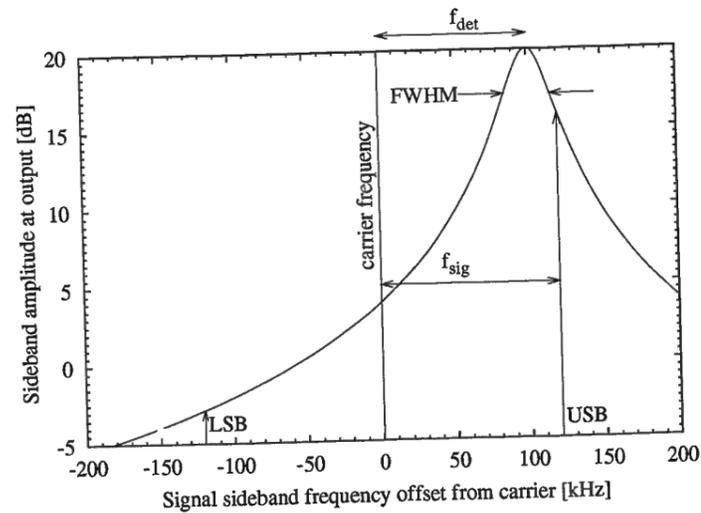
Figure 1.54: Amplitude transfer function in detuned signal recycling, using the parameters of the prototype (30 m armlength and 3.88% SR mirror transmission). The signal frequency used for the example is 120 kHz, and the frequency offset  $f_{\text{det}}$  is 100 kHz.
