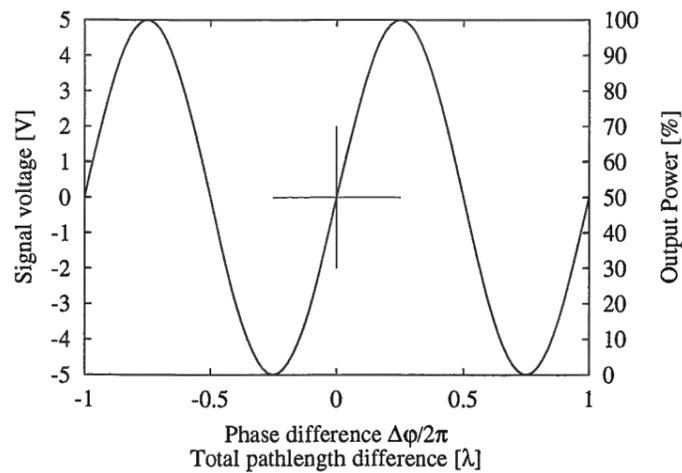
Figure A.9: Output signal of the 'mid-fringe lock' circuit shown in Figure A.8.
