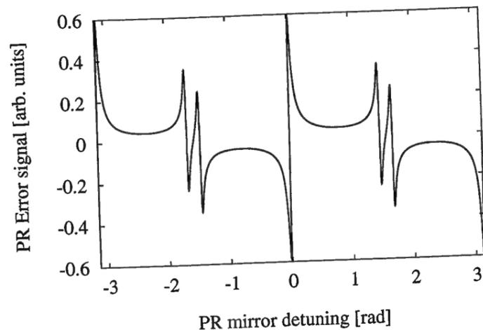
Figure 1.30: PR cavity error signal at the normal operating point.
