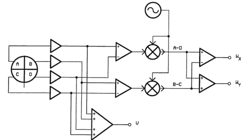
Figure 2.6: RF signal paths in the quadrant detector. The mixers are analog multipliers with differential inputs. The signal 'V' is demodulated in a separate mixer (Mix1 and Mix2 in figure A.15) and used as error signal for the Pound-Drever loop and Michelson dark fringe lock, respectively. The  $W_X$  and  $W_Y$  outputs are the error signals for the auto-alignment loops.
