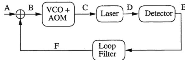
Figure A.11: Schematic of the relevant parts for the calibration of the frequency noise measurement.
