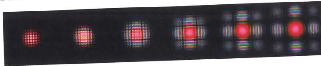
Figure 3.11: Simulation of the time of flight expansion for different evolution times. After switching off the lattice potential, a matter wave is emitted from each lattice site (left). As time evolves, the phase coherent matter waves overlap and form a multiple matter wave interference pattern. For long evolution times this pattern shows the momentum distribution with discrete momentum peaks arranged in a periodic pattern (right). This pattern corresponds to the reciprocal lattice and the Fourier transform of the wave function in the lattice. In the plot the phase of the matter wave is color coded, visualizing phase gradients as stripes.
