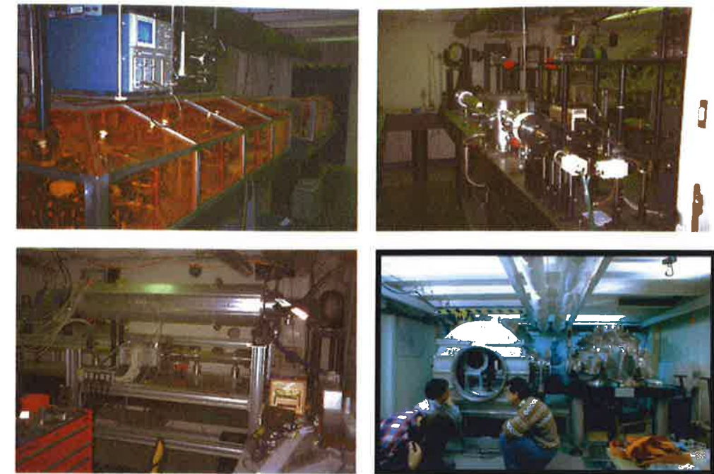
Figure 4.5: Photographs of the LULI laser system: top left: front end, top right: rod amplifier and beam diagnostics, bottom left: disc amplifier, bottom right: compressor and target chamber.
