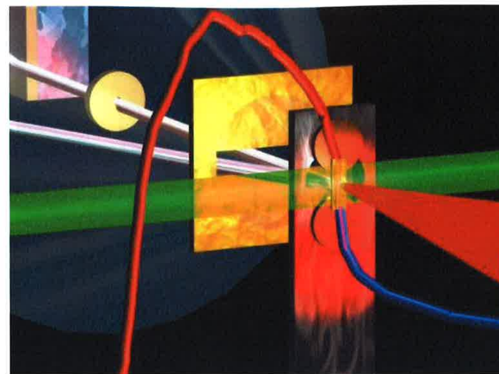
Figure 4.9: The target is mounted with free access from the front, rear and the sides. The laser is impinging on the front the ions are accelerated from the rear in laser direction where most of them hit the stack of RCF. Some pass through the slit to the spectrometers. Attached to the targets are the current-carrying wires for resistive heating.
