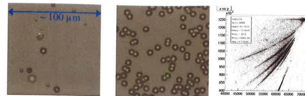
Figure 5.7: The automated scanning microscope takes a video picture and searches for tracks. Recognized tracks are fitted with ellipses and their parameters are stored. After further analysis a scatter plot reconstructs the Thomson parabola image.
