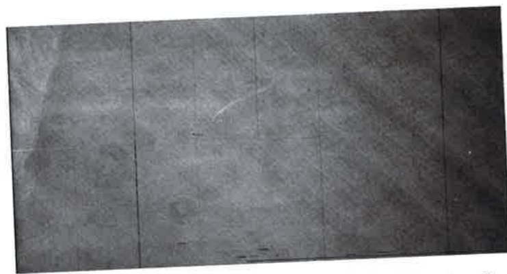
Figure 6.8 – Technical flat-field of one of the two HARPS CCDs. An altered sensitivity can be seen near the junctions between the 1024 \times 512 px wide master blocks that make up the CCD pixel array. The diagonal stripes arise from uneven device thinning during fabrication of the (back-illuminated) CCD chip.
