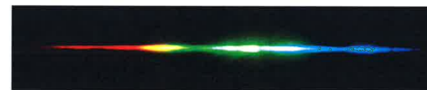
Figure 2.20 – Broadened spectrum of the 18 GHz astro-comb (no spectral flattening applied). The image represents a photograph of the astro-comb output, that was dispersed by a grating and projected on a wall (photo by R. Holzwarth).
