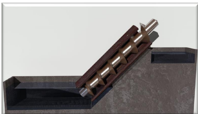
Figure 1: Archimedes screw. Continuous rotation of the screw pumps water from the lower- lying reservoir into the upper one. (Graphic: MPQ, Quantum Many Body Systems Division)
