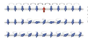
Figure 1: Illustration of the propagation of the spin impurity (red) through a chain of atoms with initially opposite spin. Graphic: MPQ, Quantum Many Body Systems Division
