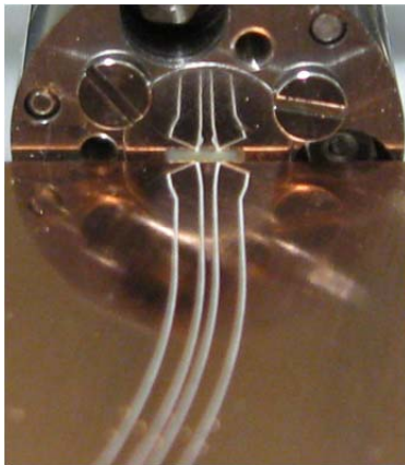
Fig. 1: Photograph of the guide with the electron source in the back. The white lines are the substrate being visible in the space between the individual electrodes. Electrons are emitted through a tiny hole of 20 \mu\text{m} diameter (not visible) in the centre of the gun. The guiding minimum forms 0.5 mm above the electrodes. Guided electrons follow the direction of the electrodes and turn to the left in the foreground of the picture.
