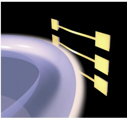
**Figure:** Schematic of the experiment: The nanostrings (yellow) interact with the optical near-field that leaks out of the toroid glass-resonator (violet). When a single string is approached into the optical near-field, the optical resonance frequency of the microresonator gets exponentially reduced.
