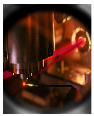
Vacuum chamber for attosecond metrology Attosecond pulses of extreme ultraviolet light (depicted as a blue beam) are focused by a mirror (right) on a jet of neon atoms effusing from a thin valve. At the same time an infrared beam is striking the atoms. Both beams in combination allow real-time observation of the motion of electrons in the neon atoms and measurement of the duration of the attosecond pulse.
