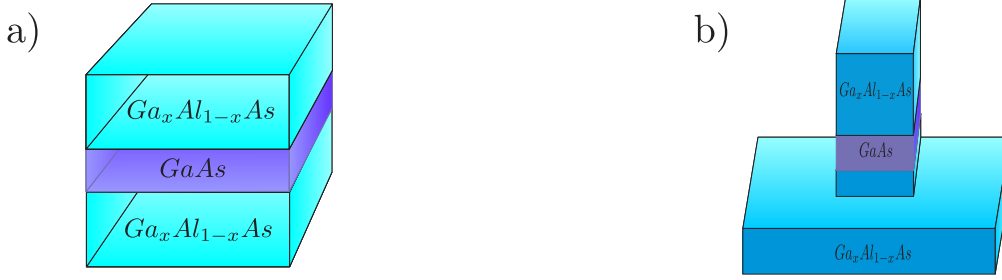
Figure 1.3: Schematic view of a) a quantum well, b) single pillar containing a quantum dot.
