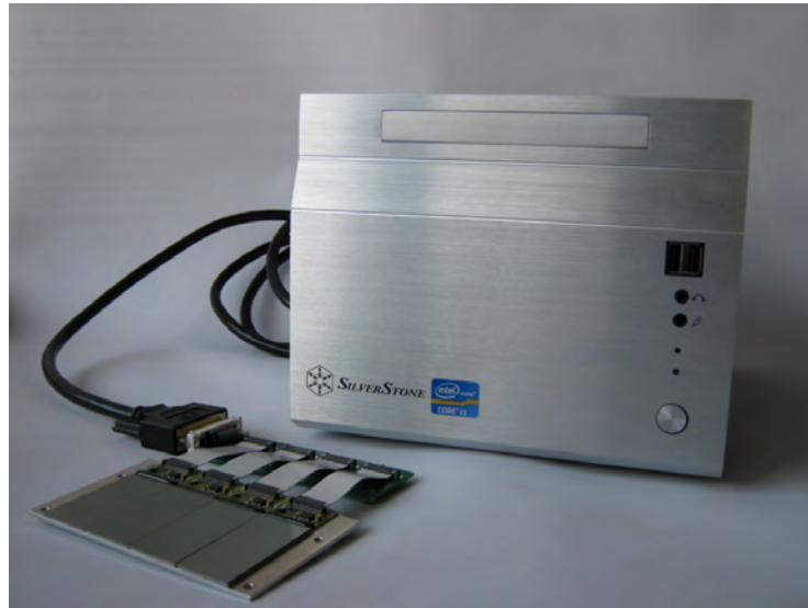
Figure 4.6: Remote RadEye detector system using four sensor modules. From Reinhardt [2012].
