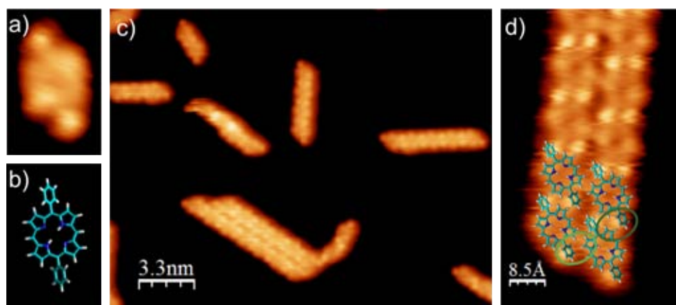
Figure 4.7: 5,15-Diphenylporphyrin on Ag(111) after RT deposition. a) High resolution STM image with b) structural model. c) Overview STM image: The molecules arrange in single or double chains. d) Double chain with structural models overlaid. The tilted phenyl rings can interact attractively with the macrocycle of a neighboring molecule. [a) 1.6 \times 2.5 \text{ nm}^2 , -0.04 \text{ V} , 0.1 \text{ nA} ; c) 23.7 \times 18.8 \text{ nm}^2 , -0.6 \text{ V} , 0.1 \text{ nA} ; d) 4.5 \times 7.6 \text{ nm}^2 , -0.05 \text{ V} , 0.7 \text{ nA} ]
