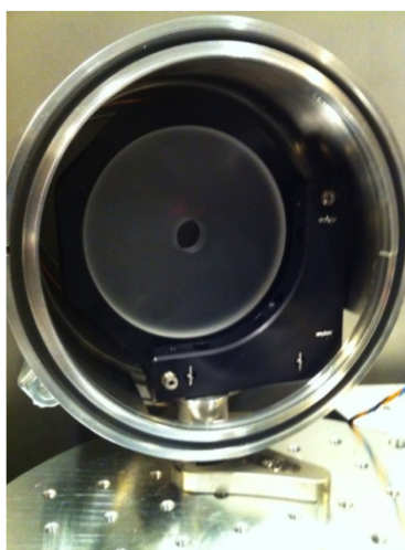
Figure 3.14: Pierced substrate for focusing the laser beam back after HHG.
