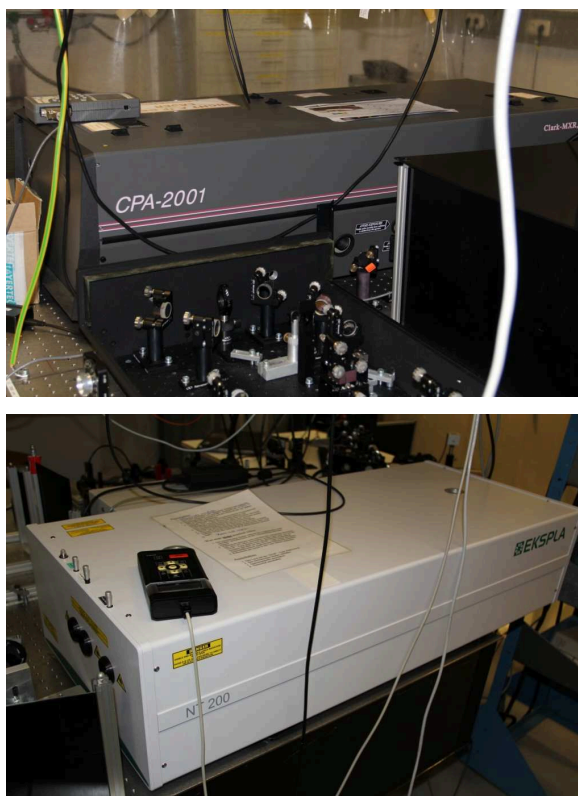
Figure A1: Regenerative Ti:Sa amplifier system (CPA 2001; Clark MXR) (top), tunable Nd:YAG laser system (NT242; EKSPLA) (bottom).
