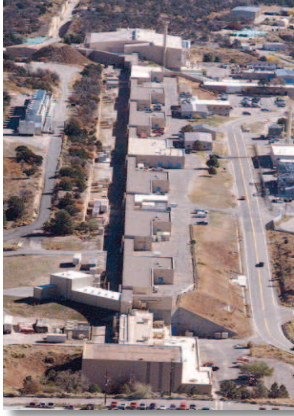
Figure 1.1: Left frame: Los Alamos Neutron Science Center (LANSCE) with its 1 km long linear accelerator to generate protons of up to 800 MeV. Middle and right frame: LANL's Trident Laser facility building and table-top front-end, where protons with 120 MeV and carbon C^{6+} ions with 1 GeV can be generated.
