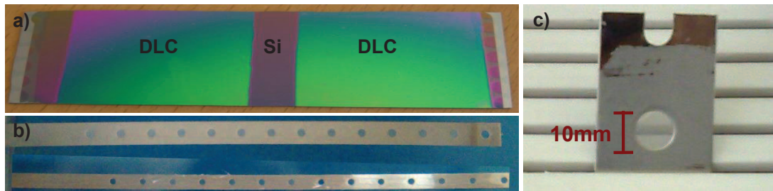
Figure 3.9: a) Picture of a silicon strip with deposited DLC; b) Typical target holder with DLC targets used in many experiments and c) 20 nm thin DLC foil free standing over a diameter of 10 mm
