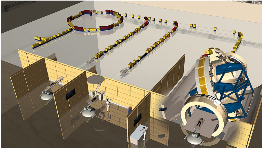
Figure 2.5: Design of the Heidelberg Ion Therapy Facility (HIT) including the synchrotron, the beam line, two fixed beam line irradiation rooms and the gantry irradiation room. The HIT-Gantry can guide heavy ions up to oxygen and rotate around 360^\circ for beam delivery. (Taken from www.klinikum.uni-heidelberg.de/Das-HIT.117970.0.html .)
