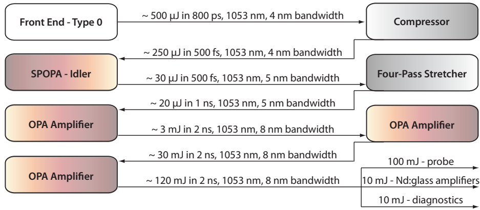
Fig. 3.10. Flow chart depiction of the revised, type 1 TRIDENT front end. The new approach relies on self-pumped optical parametric amplification (SPOPA) to generate idler pulses that are virtually background free. Those high contrast pulses are further amplified in a series of OPA stages before being sent to the Nd:glass chain.
