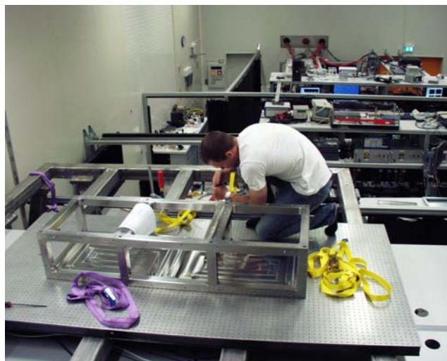
Figure A.8: Now that the bridge is safely installed, the vacuum chambers need to be put into place.
