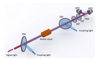
A cloud of cold atoms is illuminated with red signal light and blue coupling light. The light pulses are superimposed on dichroic mirrors (DM). With wave plates (WP), a polarizing beam splitter (PBS), and avalanche photodiodes (APD) the polarization of the transmitted signal light is determined.
