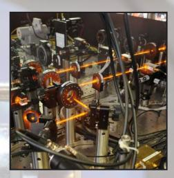
A single atom strongly coupled to a single mode of an optical resonator is a textbook example of fundamental light-matter interaction that we investigate experimentally. It allows us to observe quantum efects like photon blockade or the emission of non-classical states of light.
