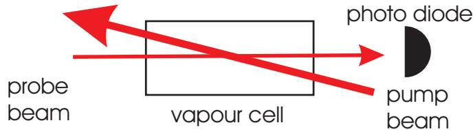
Figure 1: Basic experimental arrangement for saturation spectroscopy.
