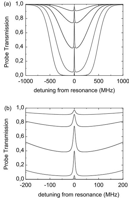
Figure 4: Probe transmission as a function of laser frequency for different vapour densities. Fig. (b) is a zoom into the region around  $\nu_0$ : for very high densities the saturated-absorption peak vanishes.
