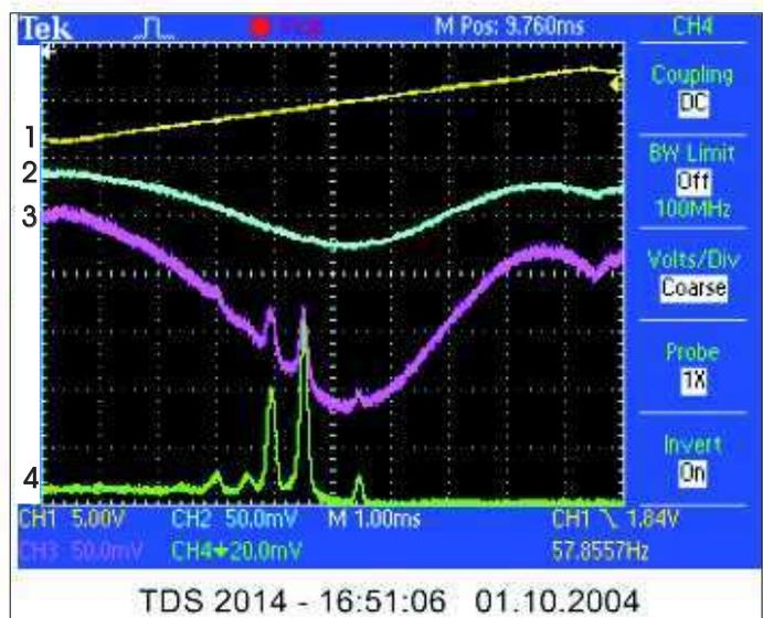
Figure 11: Oscilloscope screen shot. Yellow (1): Laser HV ramp. Blue (2): Signal of reference beam. Magenta (3): Photodiode signal of probe beam. Green (4): difference signal
