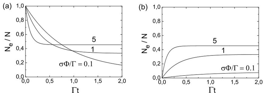
Figure 3: Excited-state population  $N_e$  as a function of time. Fig. (a) shows an exponential decay of population with  $N_e(t = 0) = N$ , in Fig. (b) the population in  $N_e$  increases exponentially in time. In any case the population in the excited state satisfies  $N_e < N/2$  for long times.
